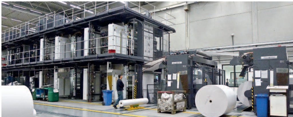
A rarity in the German newspaper landscape: the triple width, extra wide Berliner format satellite press is floor-standing. The two sets of two reelstands are positioned in front of the compact 96-page press, which has four press towers and two centrally positioned folders.
