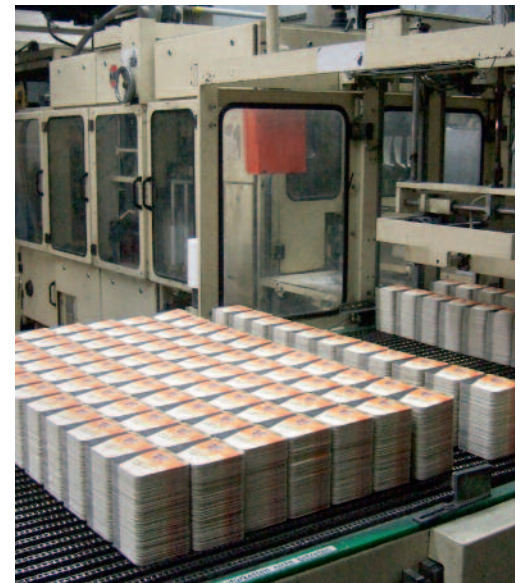
The die-cut beer mats are forwarded to the packaging machine fully automatically.
