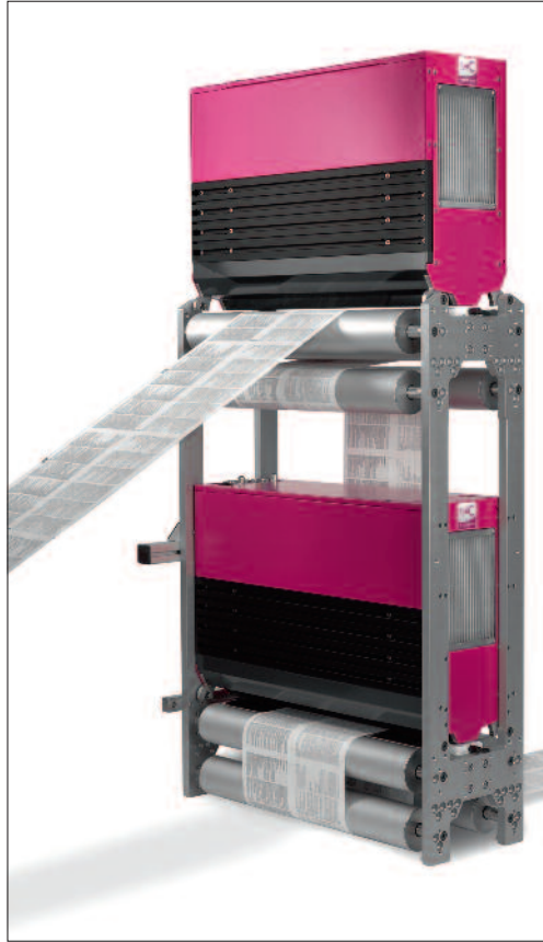
Proof-Runner in web offset printing for leaflet production at 330 m/min. (Eye-C).
