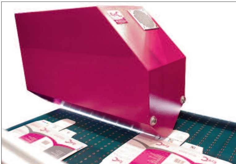
All Profiler models of the Proof-Runner Folding Carton range from Eye-C are suitable for the inspection of die-cut folding box blanks.
